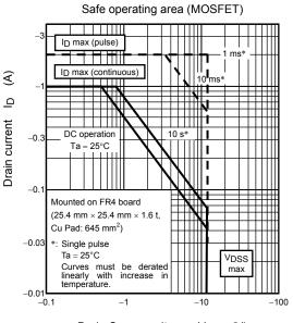
Drain-Source voltage V<sub>DS</sub> (V)
